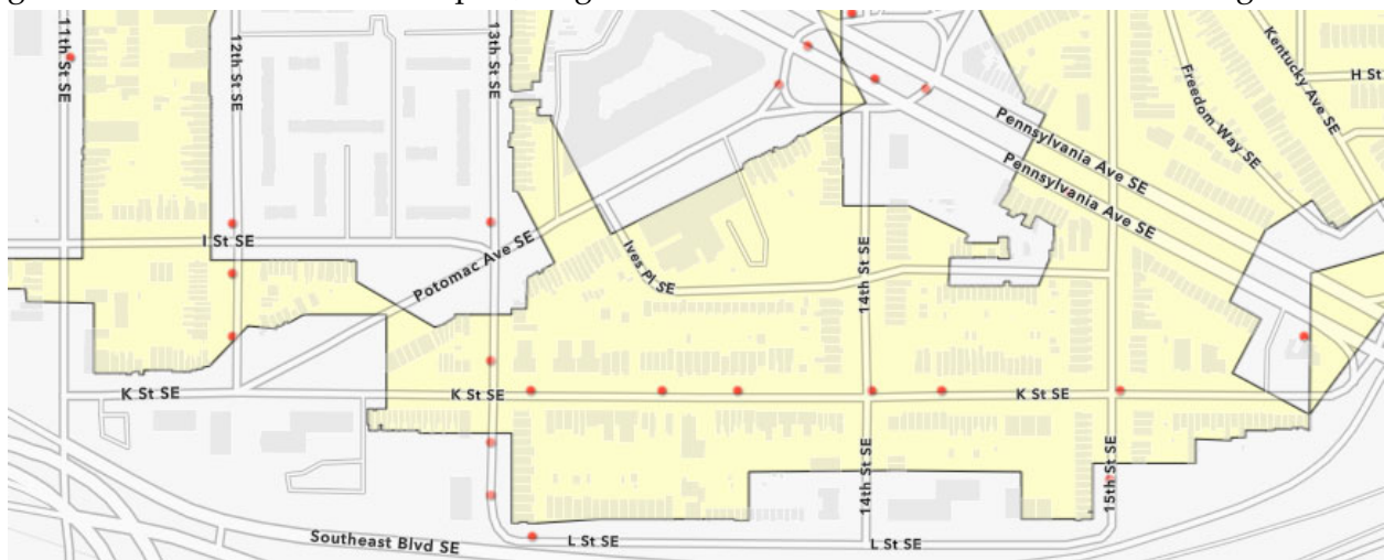
Figure 6. Capitol Hill focus area. K Street SE, was investigated in this study. Red dots indicate gas leaks detected in Phase 1 report; beige shaded areas indicated areas serviced with gas.
