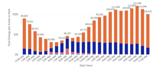
Nine (9) of the thirty-nine (39) charging stations are from ChargePoint. These charging stations are located at various commercial and multi-dwelling unit properties. Median start time for charging is 8:56AM. Based on the existing load profile, charging initiates at 5AM and peaks around 8AM and continues with higher usage until 11AM. This may coincide with EV drivers arriving at work and plugging in.
