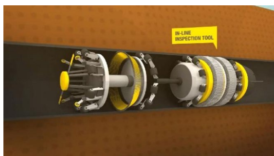
Figure 1 – Example of an in-line inspection tool in the pipe
