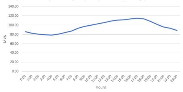
E. Representative load profile - Sample day's load profile of the system equipment.
